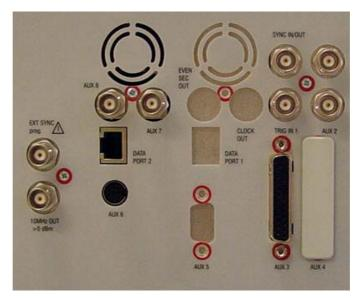
Not all of the connectors may be fitted on your 3100. The connectors actually available depend on your system configuration, in particular the installed system options.
